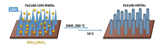
Figure 1. Synthetic process of the hybrid nanotube array FeCoNi-HNTAs.
