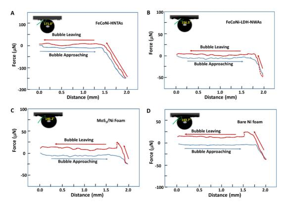
**Figure 2.** Adhesive force and contact angle measurements of gas bubbles on FeCoNi-HNTAs, FeCoNi-LDH-NWAs, MoS<sub>2</sub>/Ni Foam, and bare Ni foam.
