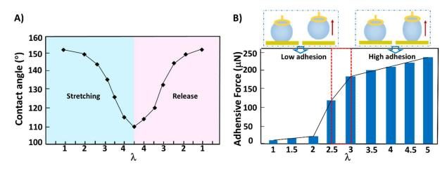
**Figure 2.** A) Reversibly tuneable surface wettability by stretching and releasing the elastomer film from  $\lambda = 1$  to  $\lambda = 4.5$ . B) Dynamic adhesion performance of the micro/nanostructured elastomer film with varying stretch ratios ( $\lambda$ ).
