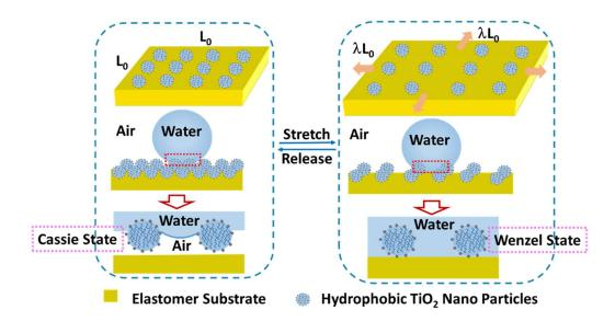
**Figure 1.** Controllable wettability of elastomer films by adjusting the space of micro/nanostructured clusters of TiO<sub>2</sub> nanoparticles on the surface through stretching.
