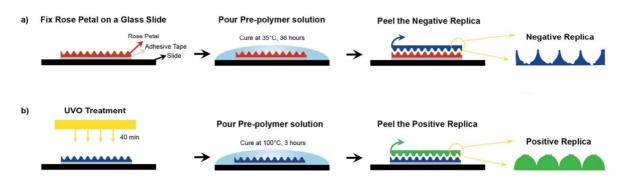
**Scheme 2:** The double molding replication technique used for fabrication of rose petal a) Negative Replica and b) Positive Replica
