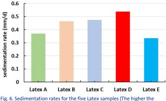
Fig. 6. Sedimentation rates for the five Latex samples (The higher sedimentation rate the less stable is the sample).
