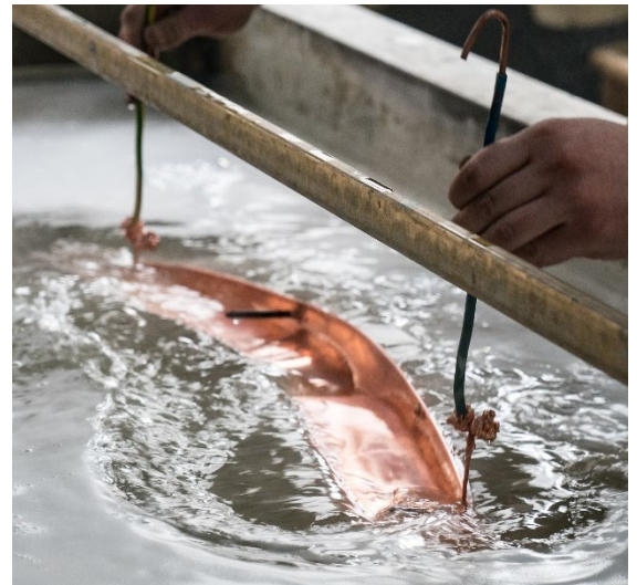
Fig. 1. Example of an electroplating bath.
