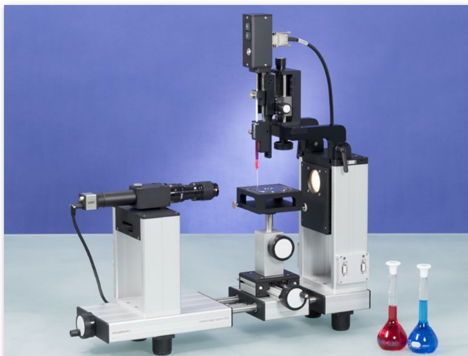
Fig. 2: Optical contact angle measuring and contour analysis system of the OCA series
