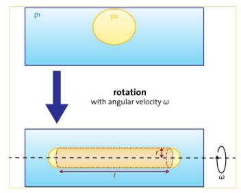
Fig. 2. Drop deformation with the spinning drop principle
