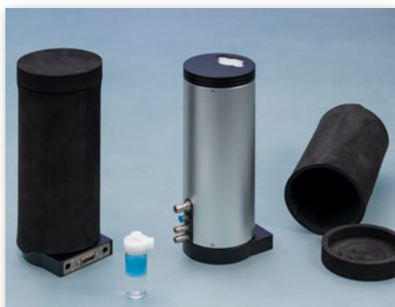
ScanTower ST-TEC with optional thermal insulation sleeve
